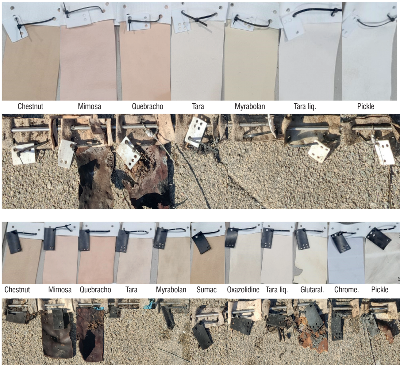
Figure 2: Samples of tanned sheep skins (top) and cow hides before and after industrial composting (50 days).
